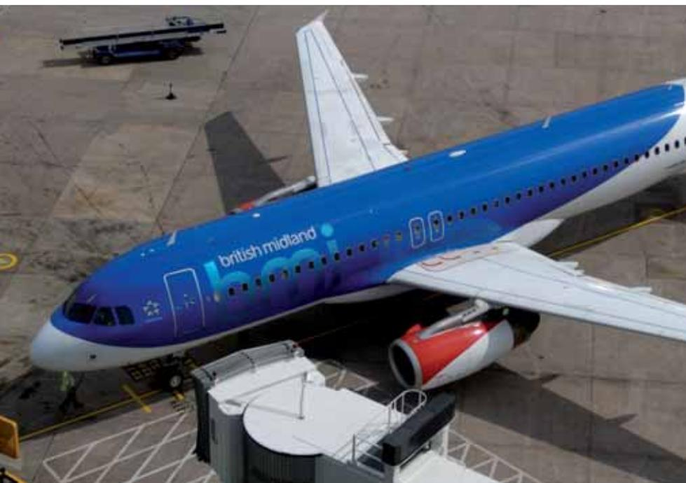
*In most cases, the V.2500 is more fuel efficient than the CFM56-5A/-5B in the order of 0.5-5%.*
