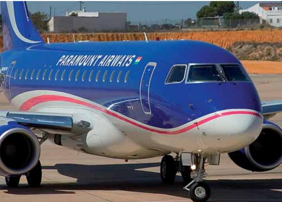
variants, is equipped with the CF34-8E rated at 14,500lbs of thrust and has a bypass ratio of 5:1.
